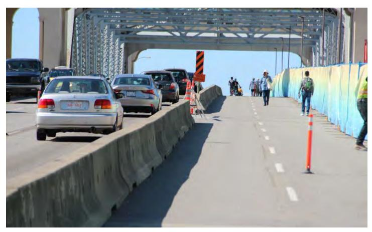
Concrete barriers provide separation from traffic on this bike lane in Vancouver, British Columbia, Canada.
