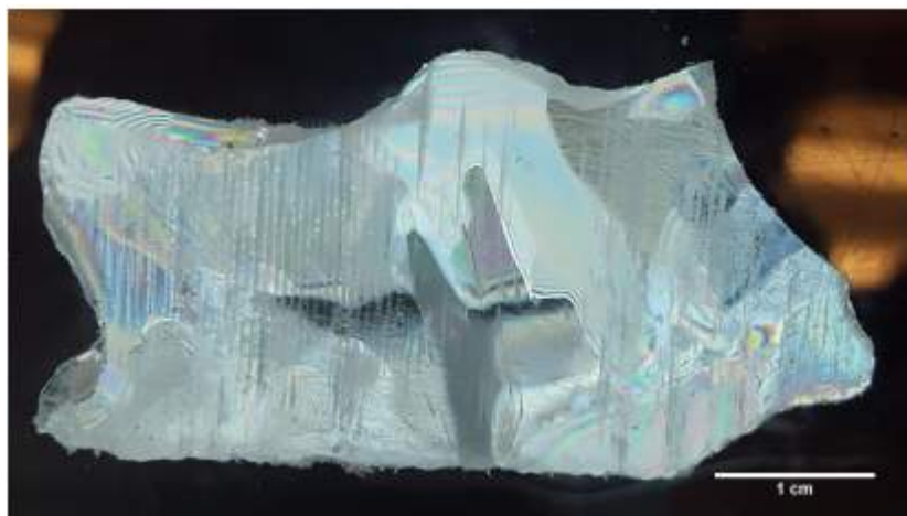
Figure 25: Section parallel to the ice-vapor interface in the bag frozen at <1 psi ambient pressure, cut from near the surface.
