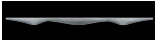
Figure 2.18: Concrete beam made with fabric formwork
