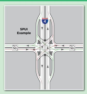
A single-point urban interchange (SPUI) is a type of interchange that is used to safely and efficiently move large traffic volumes through an intersection with limited amount of space. A SPUI allows opposing left turns to proceed simultaneously in one single intersection over or under the freeflowing road — the I-4 Ultimate project will have examples of both of these Colonial Drive will have a SPUI under I-4 and State Road 436 will have a SPUI above I-4.
