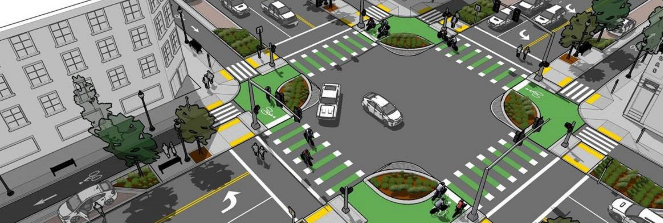
Figure 18: Protected Intersection Illustrative
