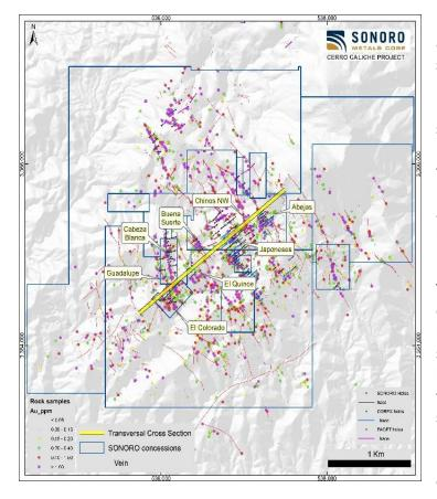
Figure 10 is a plan view of the trace of a transversal section cutting the structures contained inside Sonoro's property. The section is shown in Figure 11. The transversal section shows the pervasive character of mineralization. It is important to note areas that the not showing mineralization are a result of the absence of exploration holes, not because of an absence of mineralization.
