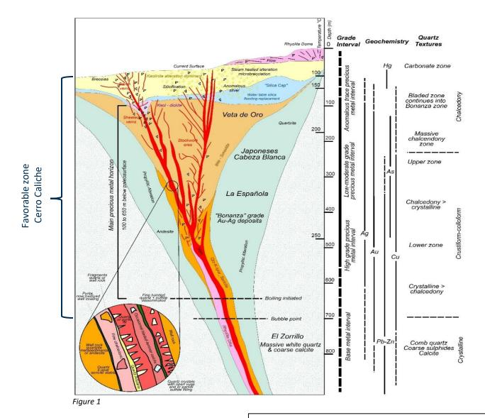
Figure 2 shows a typical longitudinal section of a LSEVS from a vein at the San Dimas Mine in the Tayoltita district, San Dimas, Durango, Mexico with the intent of indicating the extent to which these systems can develop.
