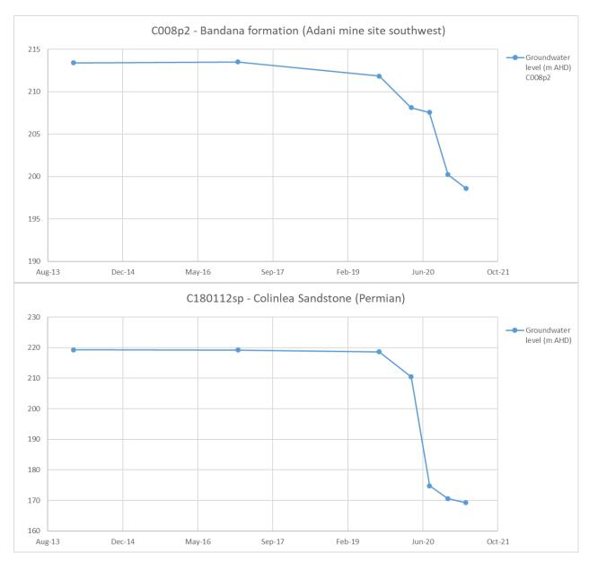
**Fig 2** – Hydrographs from 2 selected bores showing substantial drop in water levels commencing in later 2019 or early 2020, indicative of de-watering of the coal-bearing aquifer unit(s) at the Carmichael mine site. Note there is a gap in reported groundwater level monitoring data between early 2017 and mid-2019 in all bores.
