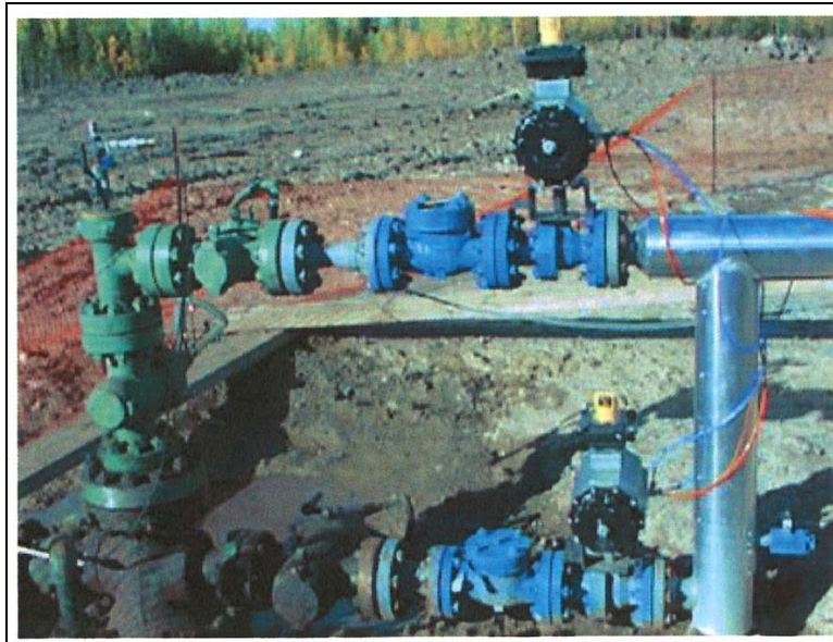
Figure 9 – Gas Wellhead with Insulation on Flow line to Protect Freezing. (Photo Courtesy of ABB Oil and Gas)
