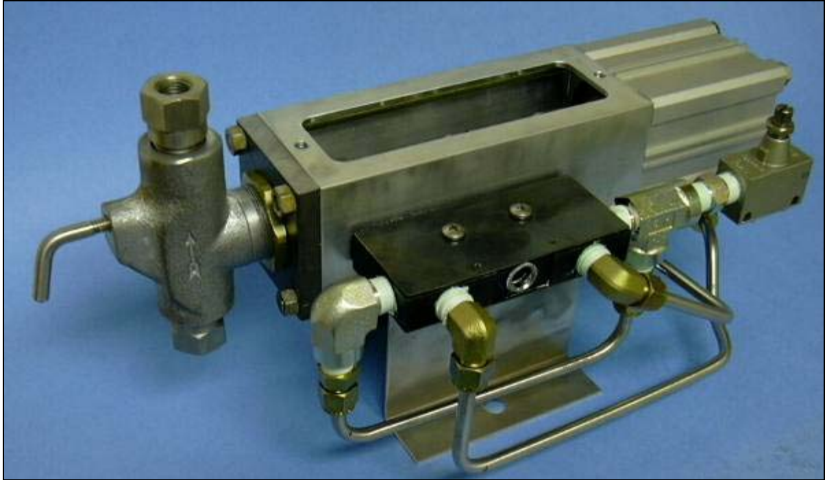
Figure 7 – Methanol Injection Pump Utilized to Inject Methanol into a Wellhead and/or Flow line to Prevent Freezing and Hydrate Buildup. Usually Located in Protected Housing on the Gas Well Location. (Ref. 11) (Photo Source ZKO Oilfield Industries; PTAC.org)
