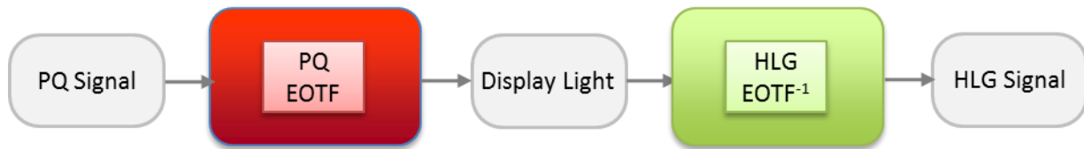
FIGURE 24 Concept of transcoding from PQ to HLG
