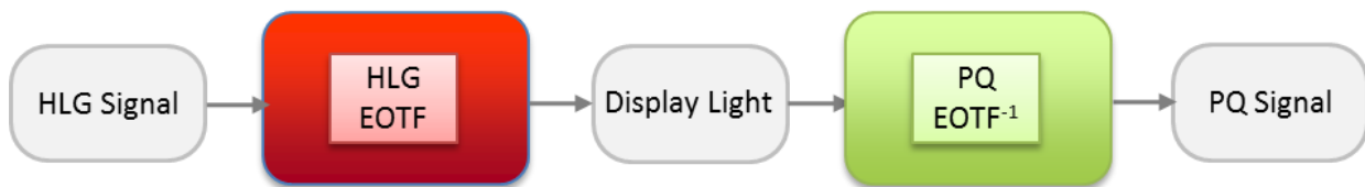
FIGURE 25 Concept of transcoding from HLG to PQ
