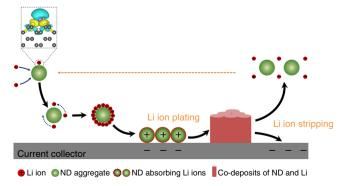
**Fig. 5** Schematic illustrating the co-deposition of Li ions on nanodiamond, growth of the columnar Li film and the stripping of Li deposits. The word "ND" in the figure is the abbreviation of "nanodiamond"
