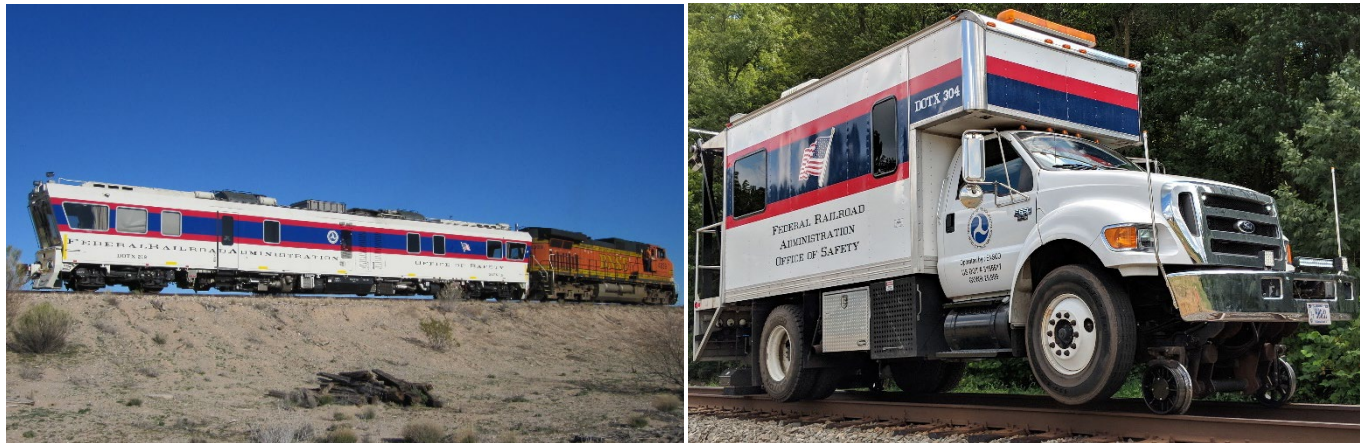
Figure 5. DOTX-219, a Staffed ATIP Track Geometry Car, and DOTX-304, a Staffed ATIP Hi-Rail Vehicle
